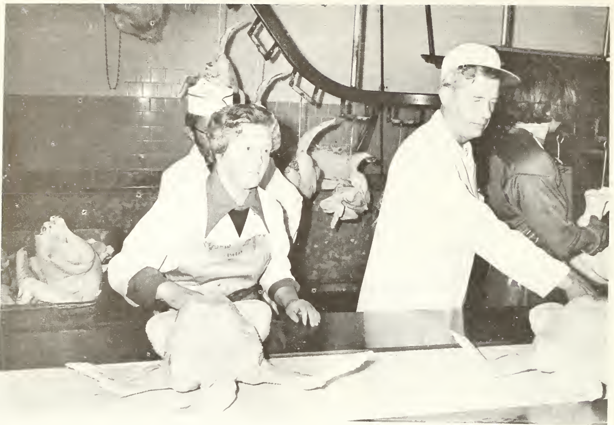
Figure 12.--Desirable work height of conveyor for short and tall graders.
